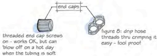
threaded end cap screws on - works OK, but can 'blow off' on a hot day when the tubing is soft.
