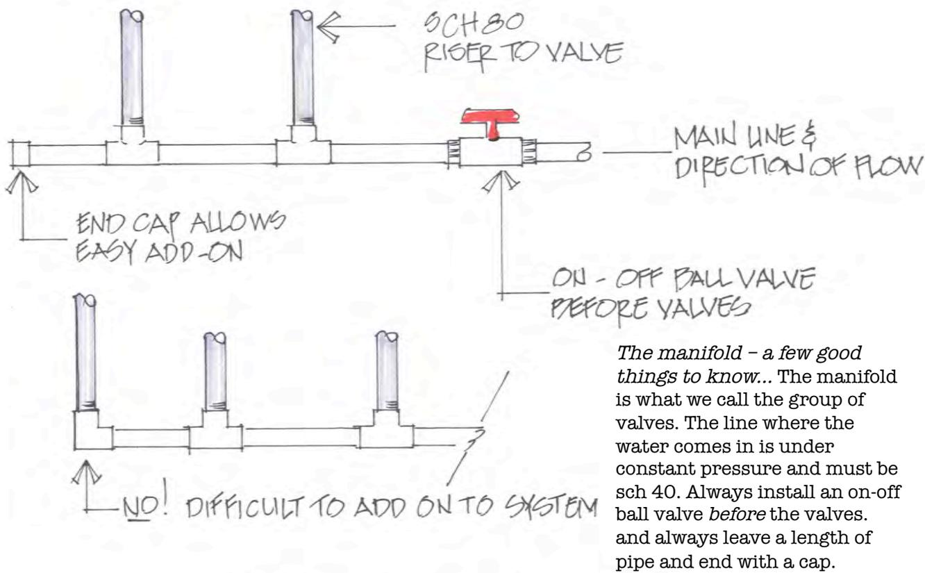
*The manifold – a few good things to know...* The manifold is what we call the group of valves. The line where the water comes in is under constant pressure and must be sch 40. Always install an on-off ball valve *before* the valves. and always leave a length of pipe and end with a cap.
