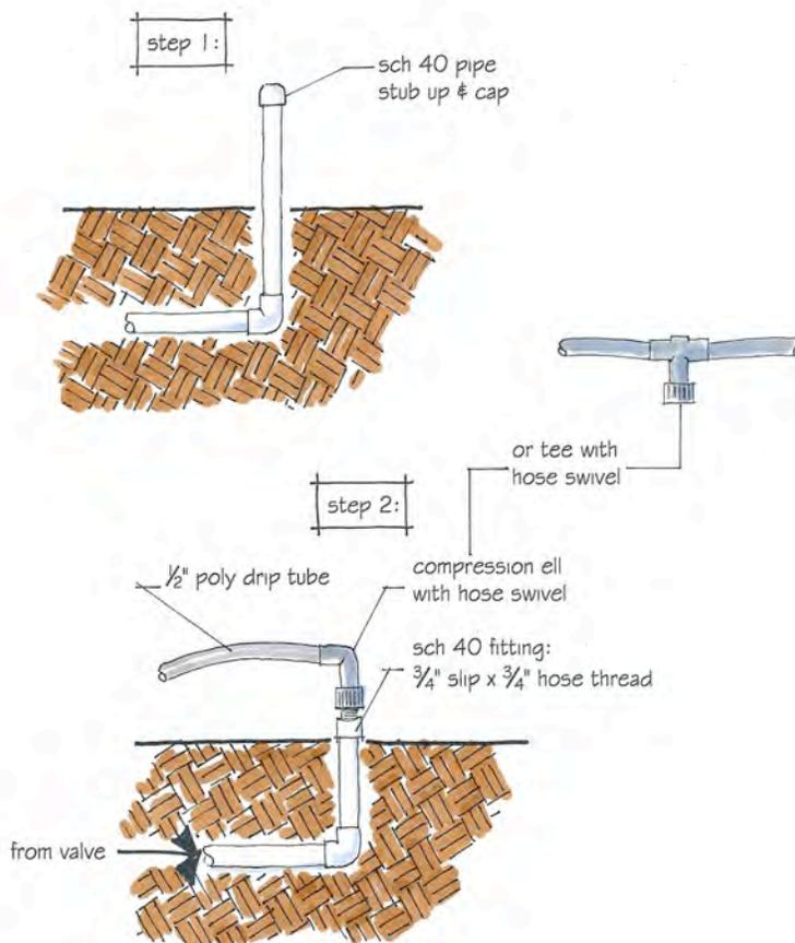
Stubbing up hard pipe – sch 40 PVC - for a new system. In step one the pipe is brought above grade and a cap is glued on, the rest of the landscape construction can continue and when final grade is achieved, the pipe is cut and a slip fitting with 3/4" MHT (male hose thread) is glued on allowing a fitting with a hose swivel to be connected: step two.
