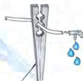
plastic hold-down to secure 1/4" drip tubing
