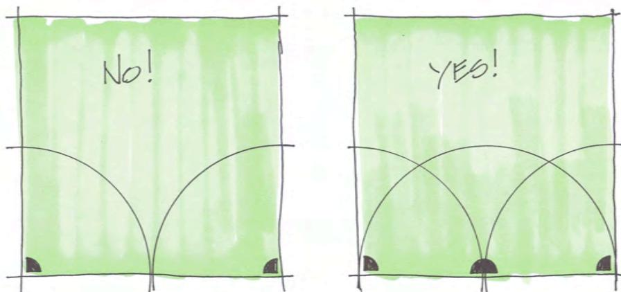
Head to head coverage means that the placement of the sprinklers allows the spray of one sprinkler (or the radius) to completely meet the head of the next sprinkler. In the illustration above the sprinklers on the left have no head to head coverage, there is no overlap, and guaranteed, in warm weather there will be brown spots in this lawn.
