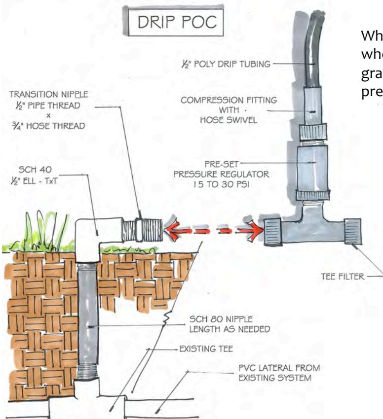
What I am calling the POC is the location where you will bring a sch 80 riser up to grade then build the assembly with filter and pressure regulator - install in order:
