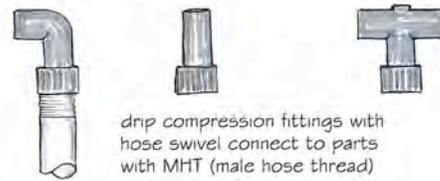
drip compression fittings with hose swivel connect to parts with MHT (male hose thread)
