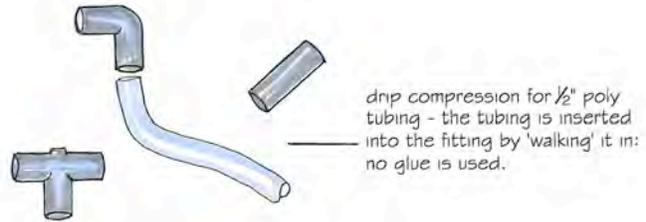
drip compression for 1/2" poly tubing - the tubing is inserted into the fitting by 'walking' it in: no glue is used.
