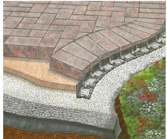
*Different edge restraints: above, a plastic type sits on top of the compacted base, below a landscape timber defines the edge and holds bricks in place.*
